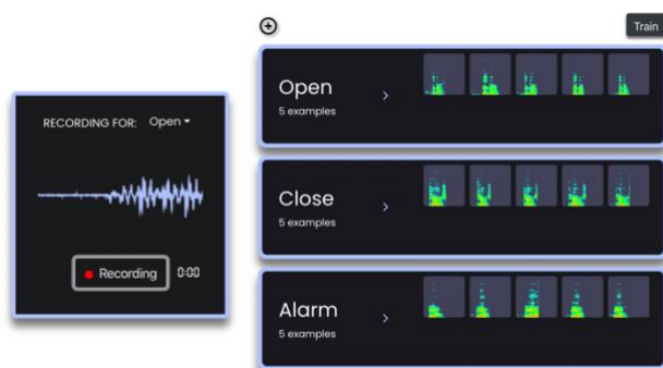
Figure 3. The label view allows users to add custom labels and record corresponding audio clips. Audio clips are up-sampled and converted to spectrograms in the browser.
